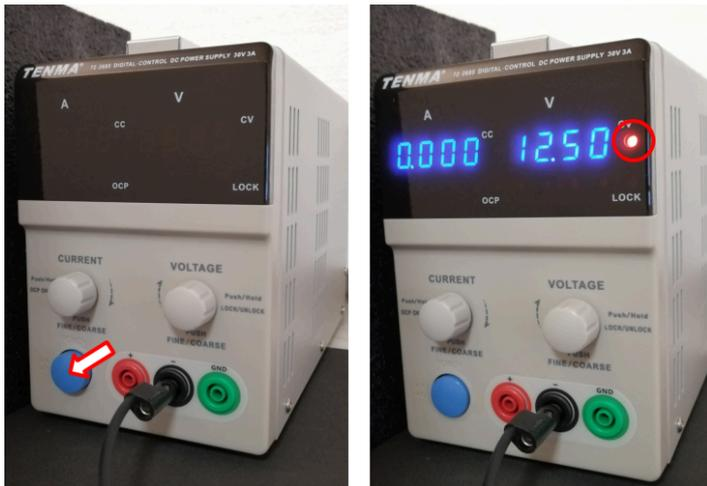
You will see two displays: current display on the left and voltage display on the right. They show the actual current and voltage at the moment, so the current will be zero, and the voltage will equal the chosen voltage limit. The CV indicator next to the voltage display will glow, indicating that the voltage limit is reached.
