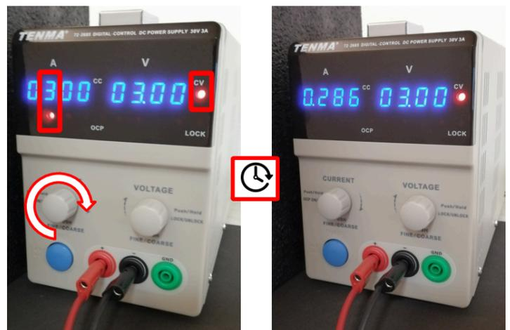
When the current is increased too much, the voltage limit is reached (CV indicator), which protects the light source. Use the current setting to control the light sources.
