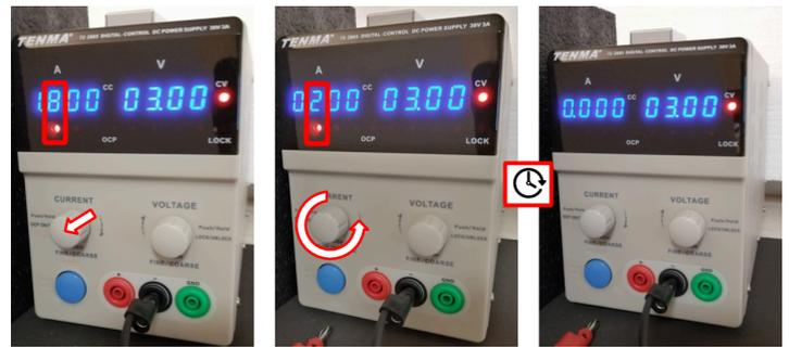
The example shows the limit 0.200 A. After 4 seconds, the display reverts to showing the actual current (still zero), and the digit selector light will turn off.
