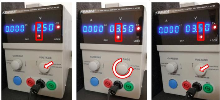
Press the voltage knob to set the voltage limit. The display will now show the voltage limit instead of the actual voltage, and the light below one of the voltage digits will glow. Turning the knob sets the chosen digit, and pressing it will cycle through all the digits. Use this to set the voltage to the maximum allowed voltage of the light source, e.g. 3.00 V for the LED.
