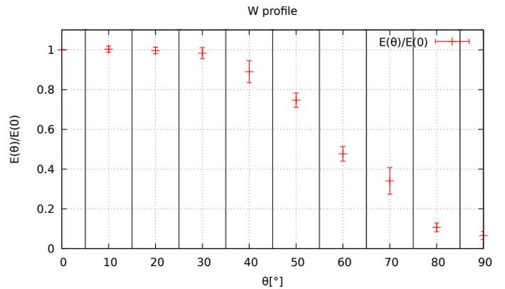
To describe the inflection point in the light distribution well, we will need at least 5 measurements in the  $\theta \in [0, \pi/2]$  interval. We can either rotate the light source on the spot, or position the light meter at different angles in relation to the stationary light source.
