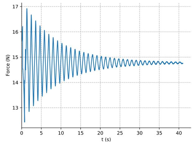
Similarly, we can amplify the larger natural frequency by oscillating the box or giving a shorter pulse.
