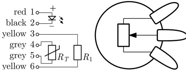
The schematic and connections of the circuit board (left) and the potentiometer (right) are in the figure. The resistor  $R_1$  may be used for heating the board near the LED. The temperature sensor (thermistor)  $R_T$  is another resistor whose resistance depends strongly on the absolute temperature  $T$ :
